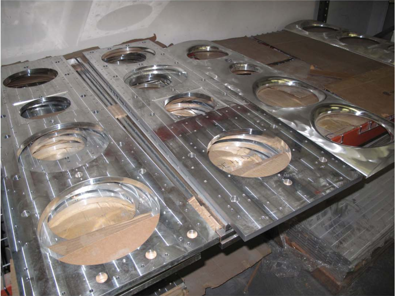
The Q7's dual baffles before polishing and anodizing. The flat baffles are on the left.
